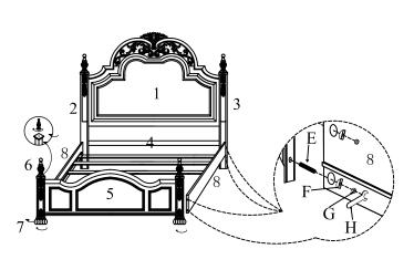
NOTE: Fasten the bolts after alignment for the bottom line of the footboard to the side rails.
