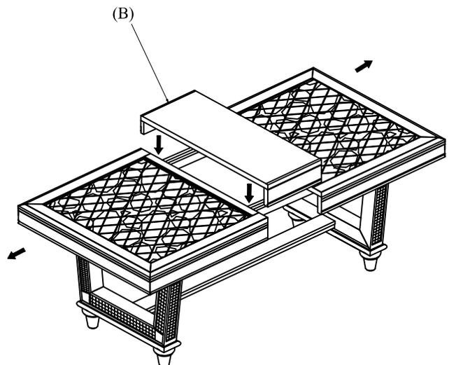
DO NOT TIGHTEN BOLTS UNTIL COMPLETELY ASSEMBLED.
