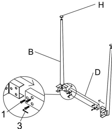
DO NOT TIGHTEN BOLTS UNTIL COMPLETELY ASSEMBLED.
