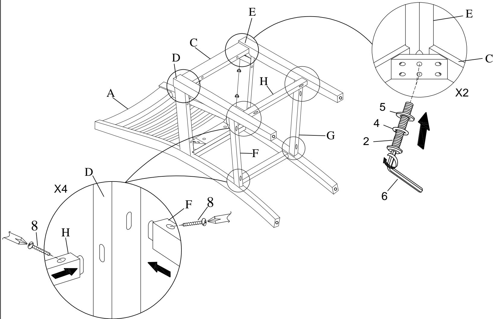
DO NOT TIGHTEN BOLTS UNTIL COMPLETELY ASSEMBLED.
