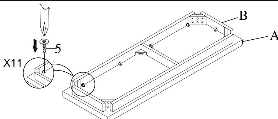
DO NOT TIGHTEN BOLTS UNTIL COMPLETELY ASSEMBLED.
