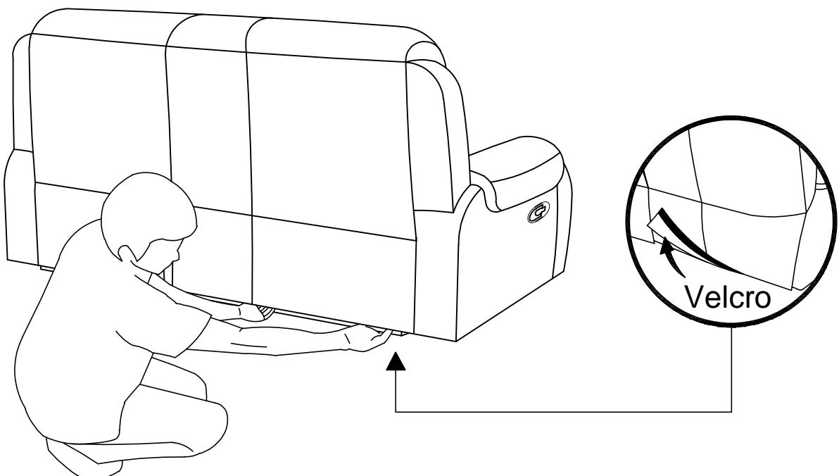
**Step #2** To unlock the back of the recliner from its base, push up on the small metal hook built into the side of the recliner
