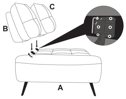
Align and push the connector to the end to lock in position properly.
