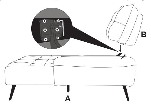
Align and push the connector to the end to lock in position properly.
