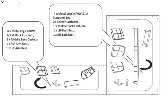
**Step 1** Align the legs to the pre-drilled holes at the bottom of the units, insert bolts and washers then tighten with Allen Key. Rotate support leg Q to tighten it.
