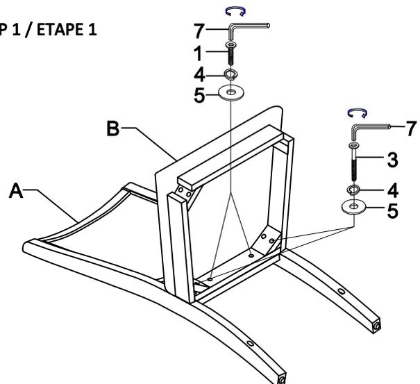
DO NOT TIGHTEN BOLTS UNTIL COMPLETELY ASSEMBLED.
