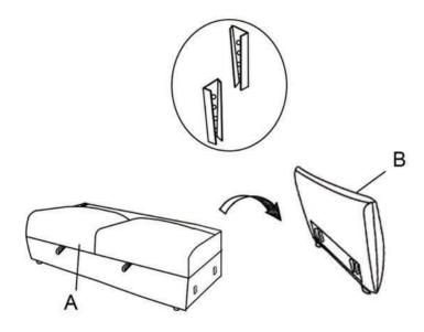
Step #3 Align and insert all brackets on back rest to seat, push to the end to secure in place properly.
