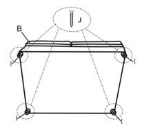
Step #3 Align and connect metal hooks to assemble the sectional.
