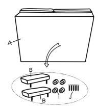
Step #2 Align legs to the pre-drilled holes, insert screws and tighten with screw driver.
