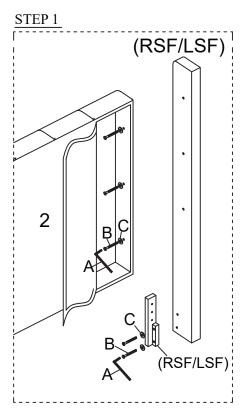
DO NOT TIGHTEN ALL THE BOLTS UNTIL COMPLETELY ASSEMBLED
