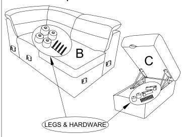
Step #2 Align the legs on the pre-drilled holes, insert screws and tighten with screwdriver(not provided).
